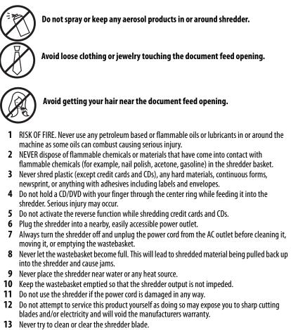
**14** Never shred beyond the specified sheet capacity. May result in extensive damage to the machine.
